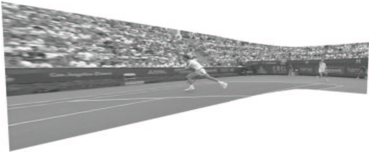
Figure 9. Sprite synthesized from Stefan sequence. Only the first 255 frames can be used since it is impossible to create the sprite for the complete sequence if the first frame is selected as reference. Sprite resolution is 2445 \times 1026 pixels.
