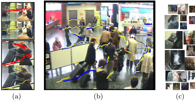
Fig. 5. (a) Tracking output (yellow lines) from tracklets (red lines). The track estimates are robust against the outliers in tracklets. (b) Tracking output (yellow lines) are compared to the ground truth (blue lines). Targets far from the camera (too small) are not tracked well. (c) Examples of false alarms by tracking. Most of them have relatively constant detection-responses, i.e. with stable appearance over time.
